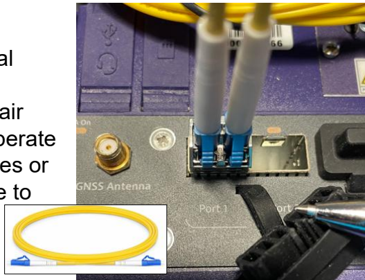
Figure 5: Insert SFP and simplex Fiber to connect Tx to Rx. Duplex example on left, BiDi on right
